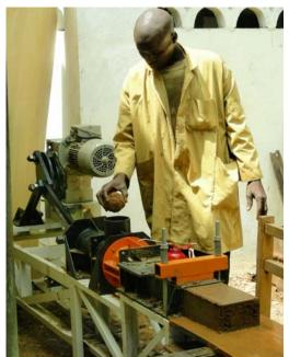
Fig. 6 - Earthen brick machine constructed in Cameroon.
