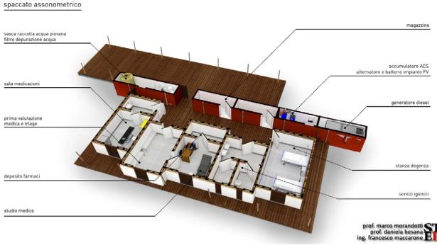
Fig. 5 - Functional layout of the dispensary unit.
