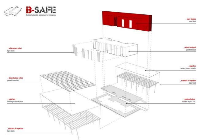
Fig. 6 - Structural schemes showing use of dry construction assembled by pallets.
